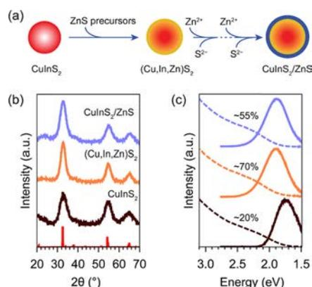
**Figure 2.** (a) Schematic diagram of the synthesis of CuInS<sub>2</sub>/ZnS QDs. (b) XRD patterns of CuInS<sub>2</sub> QDs before and after ZnS shelling. The red line indicates standard PDF card (PDF Card-01-081-9515) of the chalcopyrite CuInS<sub>2</sub>. (c) Absorption (dashed line) and PL (solid line) spectra of CuInS<sub>2</sub> QDs before and after ZnS shelling (color code is the same in panel (b)). The final product CuInS<sub>2</sub>/ZnS QDs have PLQYs of 55 ± 4%.
