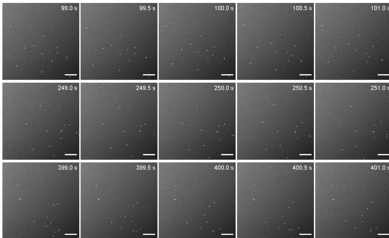
**Figure 4.** Motion of 77 nm gold NPs within the liquid-cell. The frame time was 0.5 s and frames were acquired continuously (no time between frames). The frame was  $512 \times 512$  pixels with a pixel size of 12.2 nm. The electron dose rate was  $9 \text{ e}^- \text{ nm}^{-2} \text{ s}^{-1}$ . Individual frames taken from Movie S4, Supporting Information. The scalebar is  $1 \mu\text{m}$ .
