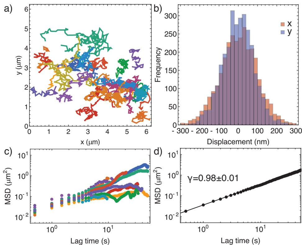
**Figure 5.** Analysis of diffusion of 77 nm gold NPs in the liquid-cell. a) First 30 tracks obtained from Movie S4, Supporting Information. b) Histogram of displacements between consecutive frames in the x- and y-directions. c) MSDs of 10 individual tracks obtained from Movie S4, Supporting Information. d) Ensemble averaged MSD from all individual MSDs in Movie S4, Supporting Information. The slope of the ensemble averaged MSD is  $0.98 \pm 0.01$ .
