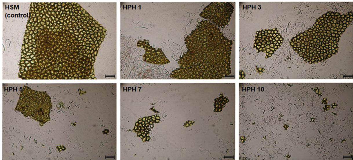
Fig. 2. Micrographs of tomato peel aqueous suspensions after HSM (control) and HPH (1, 3, 5, 7 and 10 passes) treatments. Scale bars correspond to 100 µm.
