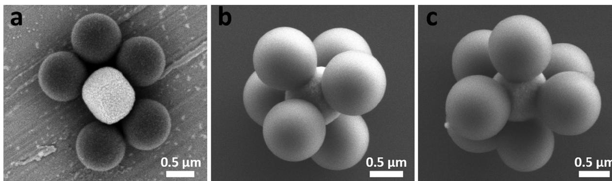
**Fig. 7.** Scanning electron microscopy images of colloidal molecules assembled from polystyrene spheres and hematite cubes. (a) Dried, unfused colloidal molecules, (b,c) Fused colloidal molecule with six and seven bound spheres, respectively.
