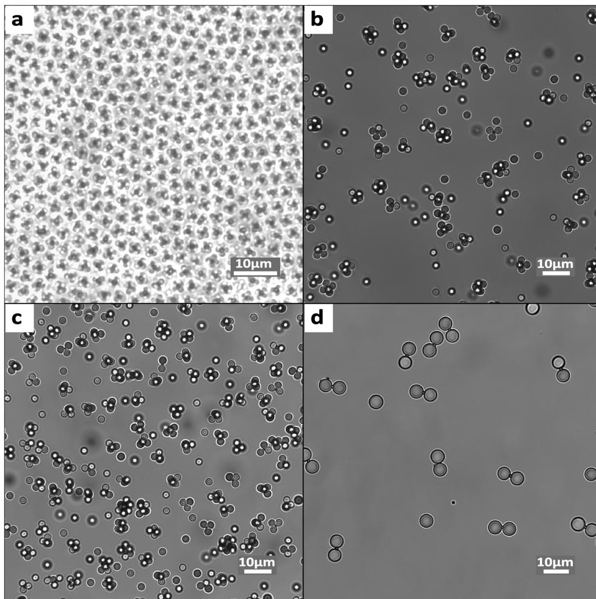
**Fig. 5.** Bright-field microscopy images of magnetically separated colloidal molecules assembled from polystyrene (PS) and hematite cubes (HC) using different size ratios  $\alpha$ : (a)  $\alpha=1.20$  assembled from PS1 and HC1, (b)  $\alpha=1.85$  (PS2 and HC2), (c)  $\alpha=2.40$  (PS2 and HC1), and (d)  $\alpha=5.48$  (PS3 and HC1).
