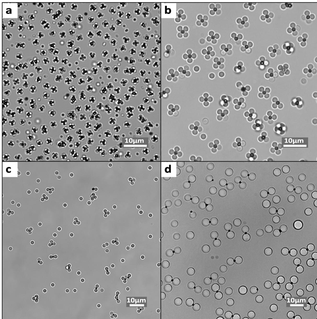
**Fig. 6.** Bright-field microscopy images of colloidal molecules assembled from silica spheres (Si1) and hematite cubes (HC) using different size ratios  $\alpha$ : (a)  $\alpha = 1.16$  (assembled from Si1 and HC1), (b)  $\alpha = 1.90$  (Si2 and HC2), (c)  $\alpha = 2.48$  (Si2 and HC1), and (d)  $\alpha = 5.56$  (Si3 an HC1).
