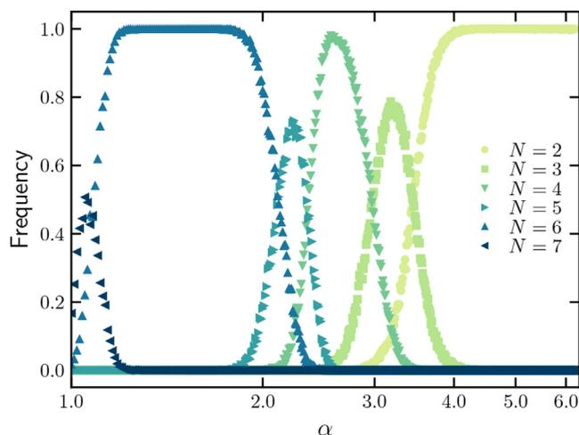
**Fig. 2.** Normalized yield of clusters with  $N$  adsorbed satellite spheres as a function of size ratio  $\alpha = \sigma_s/\sigma_c$  as obtained from Monte Carlo simulations with a repulsive screened Coulomb potential between the satellite spheres with diameter  $\sigma_s$  and an attractive screened Coulomb potential between the satellite spheres and the central cube with an edge length  $\sigma_c$ .
