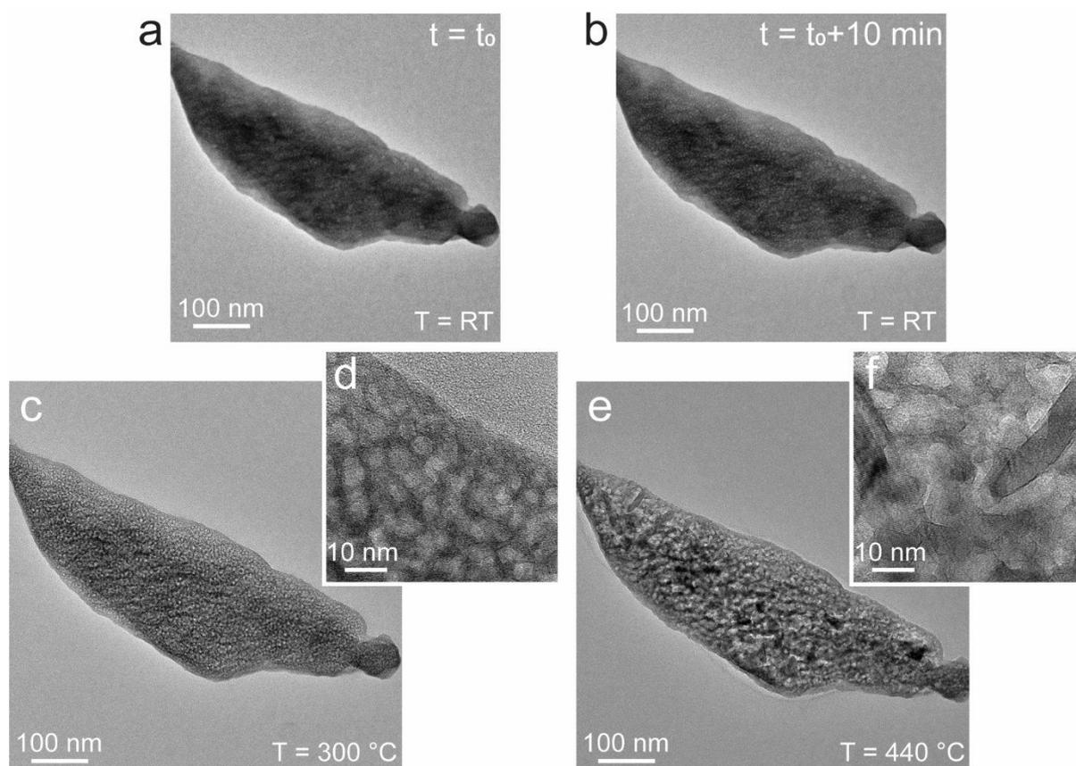
**Figure S3.** The AMV precursor was kept under the electron beam for more than 10 minutes at room temperature (a) before and (b) after exposure, not resulting in the growth of any crystalline  $V_2O_5$  nanostructures. (c & d) Images captured at 300 °C show the porous structure at the precursor. (e & f) Images captured at 440 °C show the beginning of crystallization with few already grown crystalline structures.
