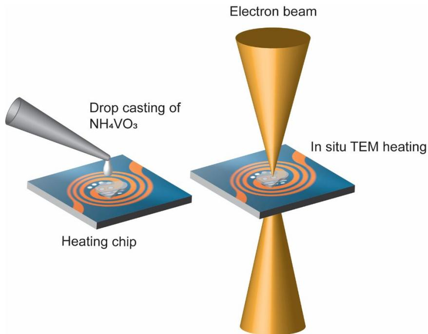
**Figure S1.** Schematic illustrating the drop-casting of ATT onto the heating chip and examination using the electron beam after the introduction of it in the TEM column for conducting the *in situ* TEM experiment.
