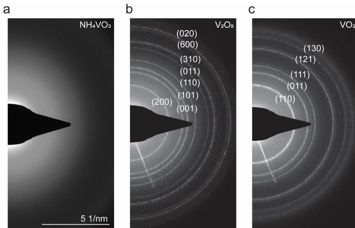
**Figure S4.** Electron diffraction patterns (DP) during the *In situ* TEM heating experiment. (a) DP of the amorphous ATT precursor at room temperature. (b) DP of the crystalline orthorhombic  $V_2O_5$  at 500 °C. (c) DP of the crystalline rutile phase  $VO_2$  at 700 °C.
