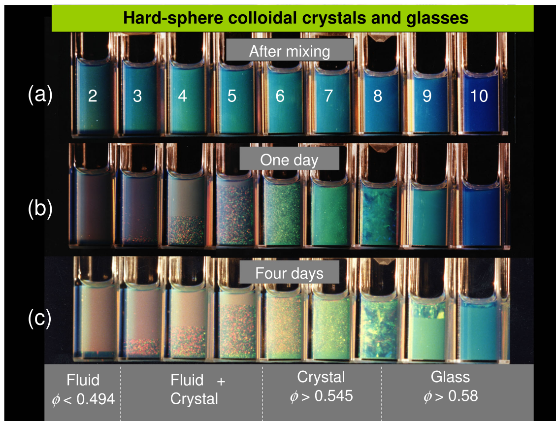
FIG. 2. The colloidal hard spheres observed by Pusey and van Megen are depicted (a) immediately, (b) one, and (c) four days after mixing. After four days, the system is presumed to have completed its phase separation. Volume fraction increases from left to right, with effective values (determined by reference to the phase behavior) \phi = 0.491, 0.517, 0.525, 0.542, 0.568, 0.593, 0.611, 0.637 , and 0.654 for samples 2–10, respectively. The samples range from a fluid phase to a fluid coexisting with an iridescent crystal; at slightly larger volume fractions the entire sample is crystalline, while at yet higher volume fractions glassy amorphous states are encountered. These states initially “coexist” with the crystal until the entire sample may ultimately crystallize. From Pusey et al. , 2009.
